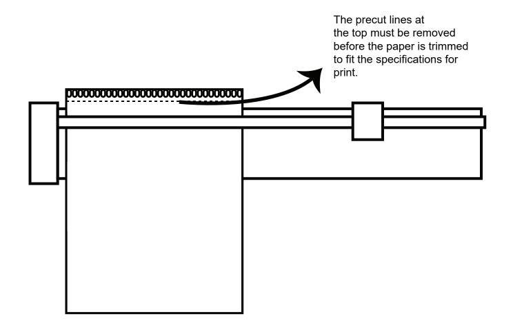
Grasp the paper trimmer blade carriage and force it to the left through the paper to cut off the excess
