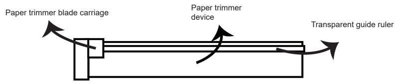
Move the paper trimmer blade carriage to the right, exceeding the maximum measurement of your to be cut paper
